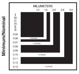
3.0 mm = 0.118 ins. 10 gauge = 0.1345/0.1225 ins. = 3.416/3.112 mm 2.5 mm = 0.098 ins. 12 gauge = 0.1046/0.0926 ins. = 2.657/2.352 mm 2.0 mm = 0.079 ins. 14 gauge = 0.0747/0.0667 ins. = 1.897/1.694 mm 1.5 mm = 0.059 ins. 16 gauge = 0.0598/0.0528 ins. = 1.519/1.341 mm
