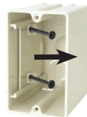
Slider plate retracted sets box in fully adjusted forward position for maximum wall substrate thickness of 1-3/8".
