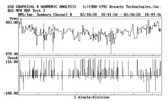
The number of surge events has jumped to well over 100, with a maximum of a positive 116.00 Vpeak and a negative of 108.00 Vpeak.
