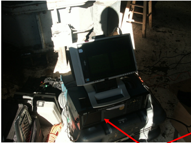
Test equipment set-up (Dranetz Power Quality Analyzer and Tablet Computer) at Drag Line 70 Lighting Panel
