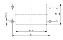
Torque for the frame's mounting screw: 2.5 – 3 Nm
